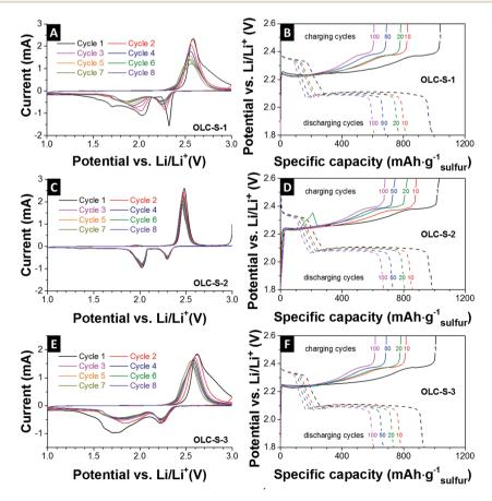
Fig. 4 Cyclic voltammograms at a rate of  $0.1 \, \text{mV} \, \text{s}^{-1}$  and galvanostatic charge—discharge curves at 336 mA  $g^{-1}$  (0.2C) for charging and 168 mA  $g^{-1}$  (0.1C) for discharging within the potential window of 1.8 V to 2.6 V *versus* Li/Li<sup>+</sup> of (A and B) OLC-S-1, (C and D) OLC-S-2, and (E and F) OLC-S-3.
