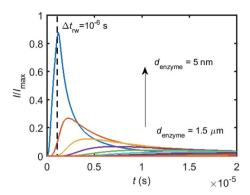
Fig. 5 Collection of the normalised current–time response to a single enzyme at a series of enzyme positions. The dashed line shows the random walk step length  $\Delta t_{\rm rw}=10^{-6}$  s. The enzyme positions  $d_{\rm enzyme}$  shown in the figure range from 5 nm to 1.5  $\mu$ m.  $r_{\rm el}=0.5~\mu$ m,  $D_{\rm P}=10^{-9}~{\rm m}^2~{\rm s}^{-1}$ .
