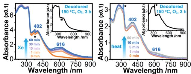
Fig. 3 (Left) Irradiated time-dependent UV-vis absorption spectra of **1** measured at room temperature in air using a 300 W Xe lamp (denoted as Xe). Inset: UV-vis spectrum after decoloration. (Right) UV-vis absorption spectra measured at room temperature in air for **1** with different thermal annealing times at 60 °C in air. Inset: UV-vis spectrum after decoloration. Noise is labelled with the \* symbol.
