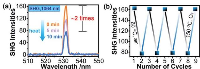
Fig. 5 (a) SHG intensity measured at room temperature in air for **1** (particle size: 150–200  $\mu\text{m}$ ; fundamental laser beam: 1064 nm, 4 mJ) with different thermal annealing times at 60 °C in air. (b) SHG-switching in four-cycle thermochromic processes. The SHG intensities are the average of one hundred single pulse signals.
