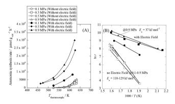
Fig. 1 Temperature and pressure dependence of ammonia synthesis activity with or without an electric field. (A) Temperature dependence of the ammonia synthesis rate at various pressures, with or without an electric field. (B) Arrhenius plots for each reaction under various pressures in the kinetic regime: catalyst bed temperature,  $463-634~\rm K$ ; catalyst,  $9.9~\rm wt\%~Cs/5.0~\rm wt\%~Ru/SrZrO_3$ ,  $200~\rm mg$ ; flow,  $N_2:H_2=60:180~\rm SCCM$ ; current,  $0~\rm or~6~\rm mA$ .
