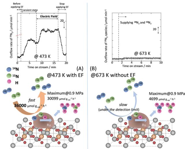
Fig. 2 Isotope exchange tests using  $^{30}\text{N}_2$ , (A) with an electric field at 473 K, and (B) without an electric field at 673 K. Catalyst, 9.9 wt% Cs/5.0 wt% Ru/SrZrO<sub>3</sub>, 200 mg; flow,  $^{28}\text{N}_2$  :  $^{30}\text{N}_2$  : H<sub>2</sub> : Ar = 6 : 6 : 36 : 12 SCCM; current, 0 or 6 mA.
