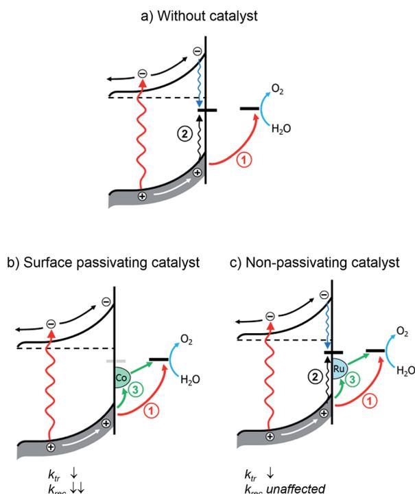
Fig. 6 Simplified model of the elementary processes in a  $\text{BiVO}_4$  photoanode (a) without a co-catalyst (b) with a surface passivating co-catalyst (e.g. CoPi) and (c) with a non-passivating co-catalyst (e.g.  $\text{RuO}_x$ ). Upon illumination, photo-excited carriers move towards the semiconductor–electrolyte interface, where direct water oxidation by valence band holes (1), surface state-mediated recombination (2), and charge transfer via co-catalyst (3) can take place.
