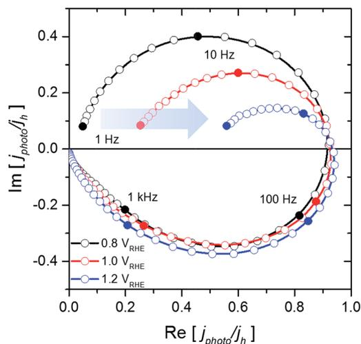
Fig. 2 IMPS spectra of  $\text{BiVO}_4$  photoanode under different applied potentials. The increase of low-frequency intercepts with increasing potential, indicate an improvement of the charge transfer efficiency.
