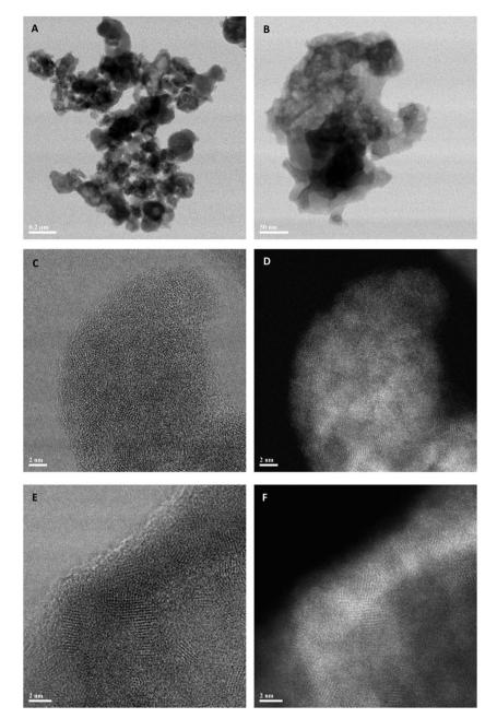
Fig. 3 Representative BF-STEM (A, B, C, E) and HAADF-STEM (D, F) images of the zincian georgeite material prepared by co-precipitation using  $(NH_4)_2CO_3$  as the precipitant.
