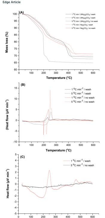
Fig. 8 (A) TGA illustrating effect of precipitation reagent, washing treatment and ramp rate on the thermal decomposition of zincian georgeite. DTA illustrating effect of ramp rate and washing treatment on the thermal decomposition of zincian georgeite prepared using (B)  $(NH_4)_2CO_3$  and (C)  $Na_2CO_3$ .
