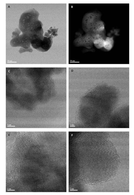
Fig. 7 Representative BF-STEM (A, C, D, E, F) and HAADF-STEM (B) images of the zincian georgeite material prepared by co-precipitation using  $(NH_4)_2CO_3$  after calcination at 300 °C.
