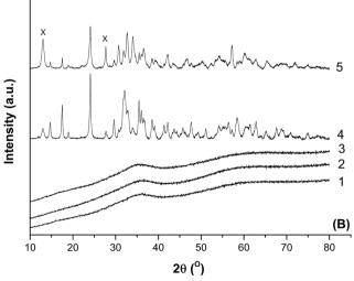
Fig. 1 (A) FT-IR spectra and (B) XRD patterns of 2:1 Cu: Zn hydroxyearbonates prepared at 40 °C using metal acetates and (1) (NH<sub>4</sub>)<sub>2</sub>CO<sub>3</sub> (2)  $NH_4HCO_3$  or (3)  $Na_2CO_3$ . Metal nitrates and  $Na_2CO_3$  were also used to prepare hydroxycarbonates at 65 °C with Cu: Zn molar ratios of (4) 2:1 and (5) 1:1. For clarity, metal acetate bands (\*) and aurichalcite bands/reflections (X) are marked
