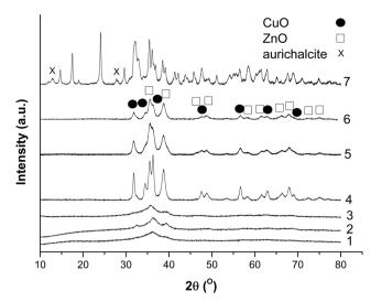
Fig. 6 XRD patterns of the calcined zincian georgeite materials prepared using: (1)  $(NH_4)_2CO_3$  (washed), (2)  $(NH_4)HCO_3$  (washed), (3)  $Na_2CO_3$  (washed), (4)  $(NH_4)_2CO_3$  (no wash), (5)  $(NH_4)HCO_3$  (no wash), and (6)  $Na_2CO_3$  (no wash). For comparative purposes, the calcined zincian malachite/aurichalcite material (7) is also presented. All unmarked reflections are associated with the zincian malachite or aurichalcite phases.
