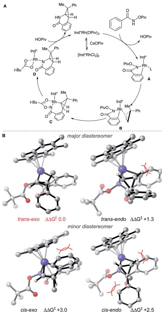
Scheme 2 (A) Proposed reaction mechanism and (B) stereochemical model for diastereoselectivity. Gibbs energies in kcal mol<sup>-1</sup>.
