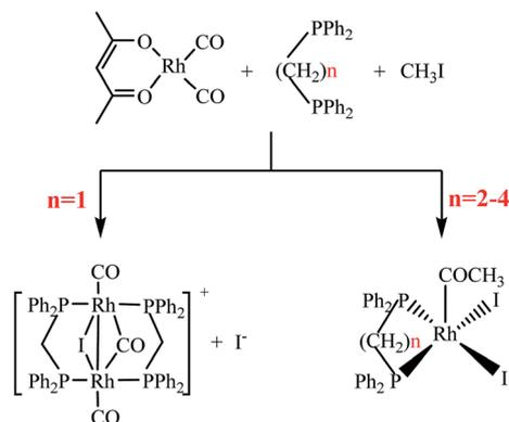
**Scheme 1** Synthetic pathways of Rh–diphosphine complexes *via* reaction of rhodium precursor with methyl iodide and diphosphine ligands ( $\text{Ph}_2\text{P}(\text{CH}_2)_n\text{PPh}_2$ ,  $n = 1-4$ ). Byproducts of CO and 4-methoxy-3-penten-2-one are not included for the sake of clarity.
