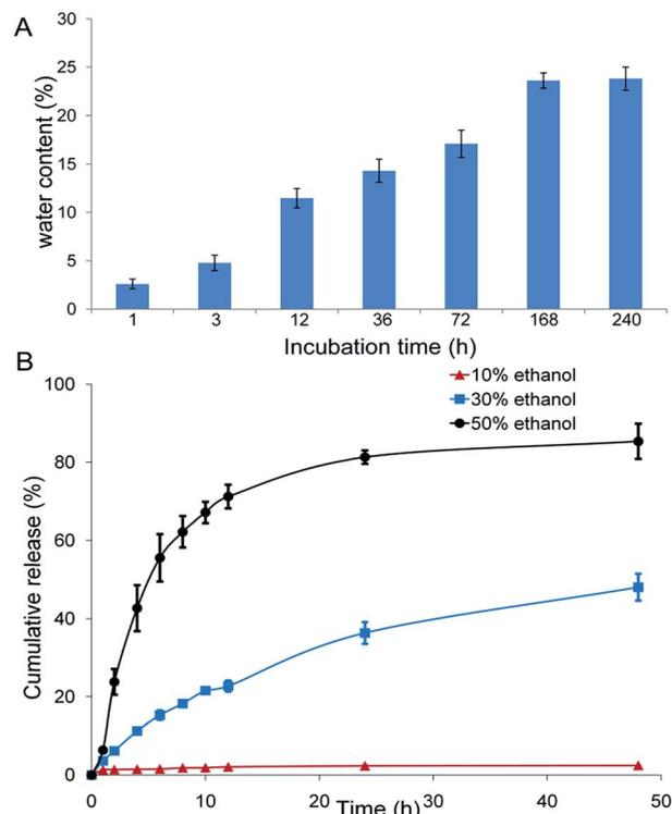
Fig. 3 Water content of DABE-LPTS and *in vitro* release of DABE. (A) Water content of DABE-LPTS after incubation in PBS (pH 7.4). Data are mean  $\pm$  SD ( $n = 3$ ). (B) *In vitro* release profiles of DABE from DABE-LPTS in release media containing 10, 30 or 50% of ethanol (v/v) in PBS (pH 7.4). Data are mean  $\pm$  SD ( $n = 3$ ).
