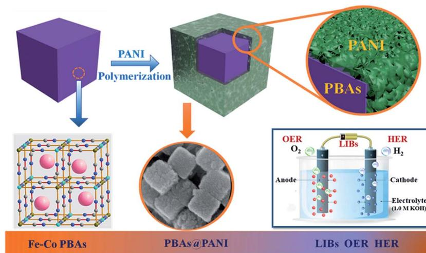
**Scheme 1** Schematic illustration of the formation process of PBAs@PANI core-shell structure, starting from the open-framework of Fe-Co PBAs. The PANI shell was coated on the surface of PBAs nanocubes *via in situ* chemical oxidative polymerization. The resultant PBAs@PANI was applied as anode material for LIBs and bifunctional electrocatalysts for overall water electrolysis.
