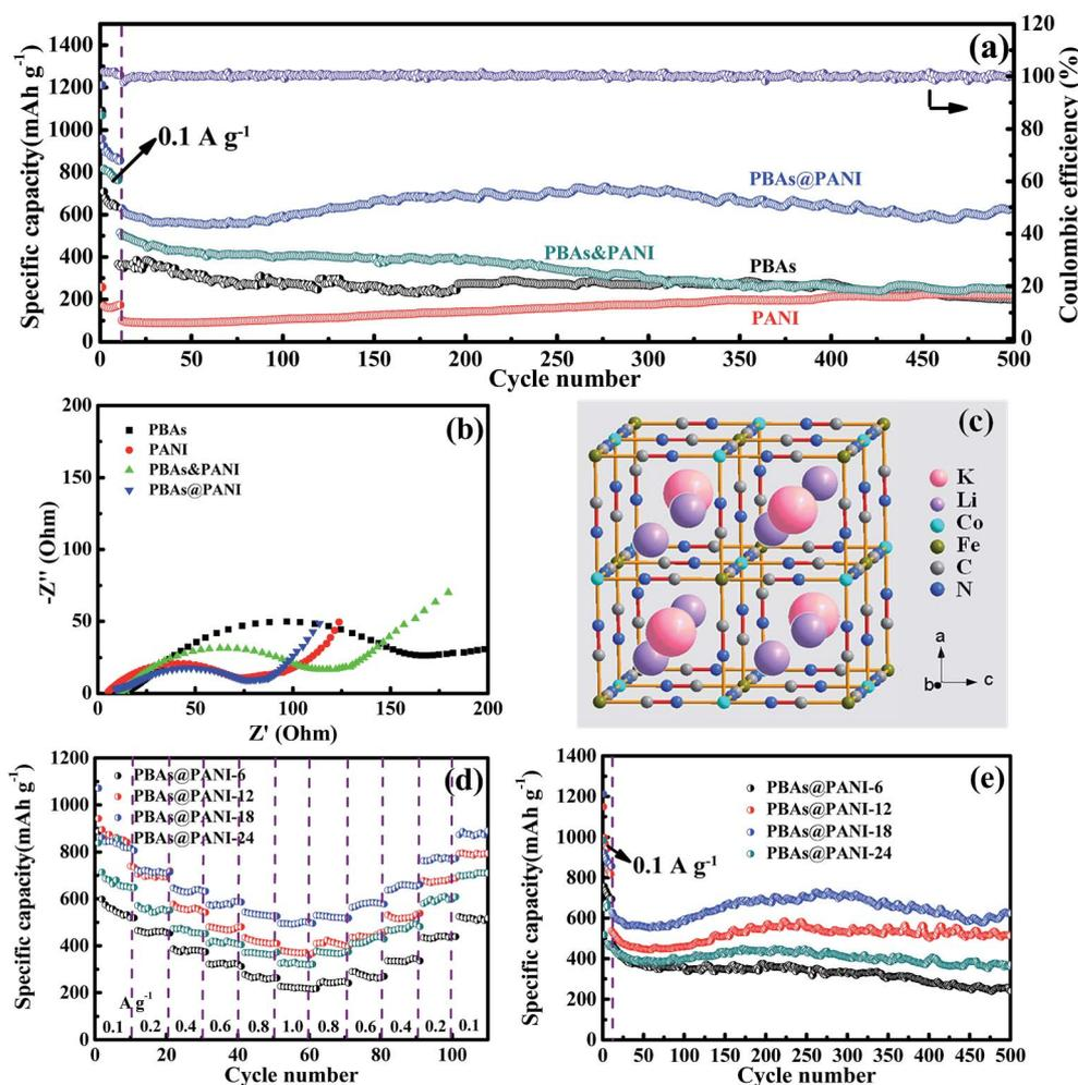
Fig. 5 (a) Long cycling performances of PBAs@PANI, bare PBAs, pure PANI and PBAs&PANI at  $1 \text{ A g}^{-1}$  after activation at  $0.1 \text{ mA g}^{-1}$  for initial ten cycles. (b) Nyquist plots of PBAs@PANI, bare PBAs, pure PANI and PBAs&PANI. (c) Schematic illustration of the insertion of lithium ions into the Fe–Co PBAs. (d) Rate and (e) long cycling performances for a series of PBAs@PANI at  $1 \text{ A g}^{-1}$  after activation at  $0.1 \text{ A g}^{-1}$  for initial ten cycles.
