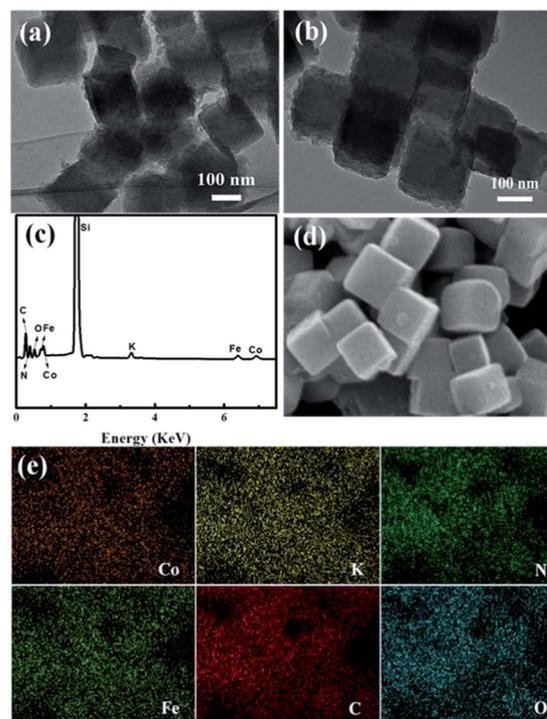
Fig. 2 (a, b) TEM images of PBAs@PANI after 18 h polymerization. (c) EDS spectrum, (d) FE-SEM image and (e) corresponding elemental mappings of PBAs@PANI.
