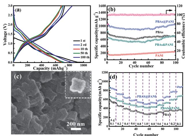
Fig. 4 (a) Galvanostatic charge/discharge profiles of PBAs@PANI at a current density of  $100\text{ mA g}^{-1}$  between  $0.01$  and  $3.0\text{ V}$ . (b) Cycling performances of PBAs@PANI, bare PBAs, pure PANI and PBAs@PANI at a current density of  $100\text{ mA g}^{-1}$ . (c) FE-SEM images of PBAs@PANI electrode after being tested for 100 cycles at a current density of  $100\text{ mA g}^{-1}$ . (d) Rate performances of PBAs@PANI, bare PBAs, and PBAs@PANI at different current densities.
