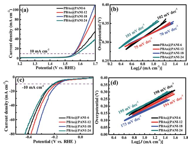
**Fig. 8** (a) Polarization curves and (b) Tafel plots of a series of PBAs@PANI for OER in an O<sub>2</sub>-saturated 1.0 M KOH solution (scan rate of 5 mV s<sup>-1</sup>). (c) Polarization curves and (d) Tafel plots of a series of PBAs@PANI for HER in an N<sub>2</sub>-saturated 1.0 M KOH solution (scan rate of 5 mV s<sup>-1</sup>).
