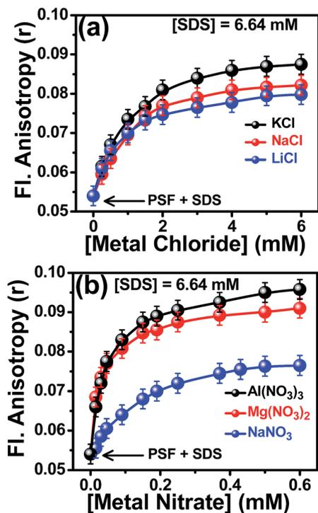
Fig. 5 Variation of the fluorescence anisotropy ( $r$ ) of SDS-bound PSF as a function of concentrations of (a) chloride salts with same valencies of the cations and (b) nitrate salts with variable valencies of the cations. The added salts are mentioned in the legends.
