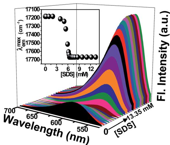
Fig. 1 Emission spectra of PSF in the presence of different SDS concentrations. Inset shows the variation of respective fluorescence maxima against the SDS concentrations. [PSF] = 5  $\mu$ M,  $\lambda_{exc}$  = 520 nm.
