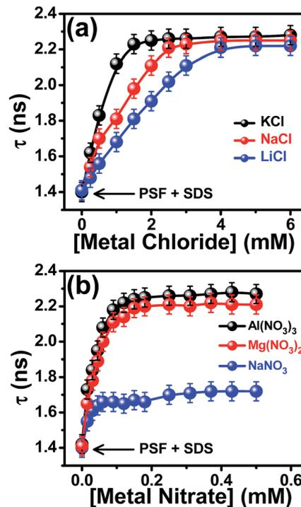
Fig. 7 Variation of the fluorescence lifetime ( $\tau$ ) of SDS-bound PSF as a function of concentrations of (a) chloride salts with same valencies of the cations and (b) nitrate salts with variable valencies of the cations. The added salts are mentioned in the legends. [SDS] = 6.64 mM. For details see text.
