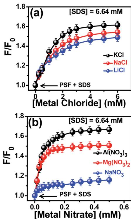
Fig. 4 Variation of the relative fluorescence intensities ( $F/F_0$ ) of SDS-bound PSF as a function of concentrations of (a) chloride salts with same valencies of the cations and (b) nitrate salts with variable valencies of the cations. The added salts are mentioned in the legends.
