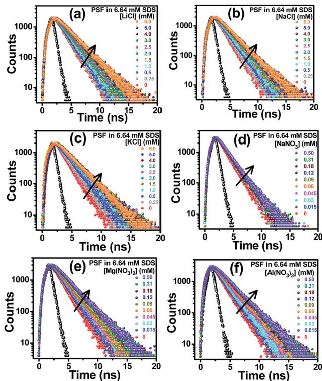
Fig. 6 Time resolved fluorescence decay profiles of PSF in 6.64 mM SDS in the presence of different concentrations of (a) LiCl (b) NaCl, (c) KCl, (d) NaNO<sub>3</sub>, (e) Mg(NO<sub>3</sub>)<sub>2</sub> and (f) Al(NO<sub>3</sub>)<sub>3</sub>. Legends give concentrations of the added salts. The sharp black profiles on the left represent the instrument response function (IRF).  $\lambda_{\text{exc}} = 490 \text{ nm}$  and  $\lambda_{\text{em}} = \lambda_{\text{em}}^{\text{max}}$ .
