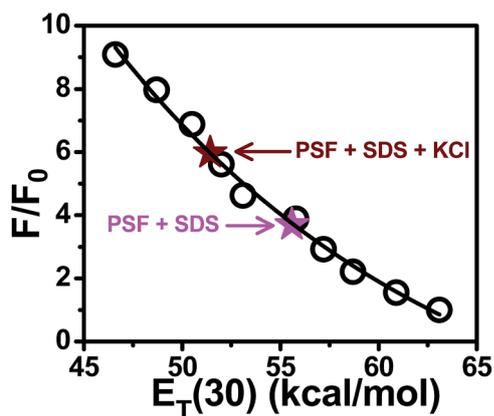
Fig. 8 Plot of variation of the relative fluorescence enhancement of PSF as a function of  $E_T(30)$  in dioxane–water solvent mixtures.  $F_0$  represents the fluorescence intensity in pure water. The magenta and the wine points are the interpolated relative fluorescence intensities in 6.64 mM SDS solution in the absence and in the presence of 6 mM KCl salt respectively.
