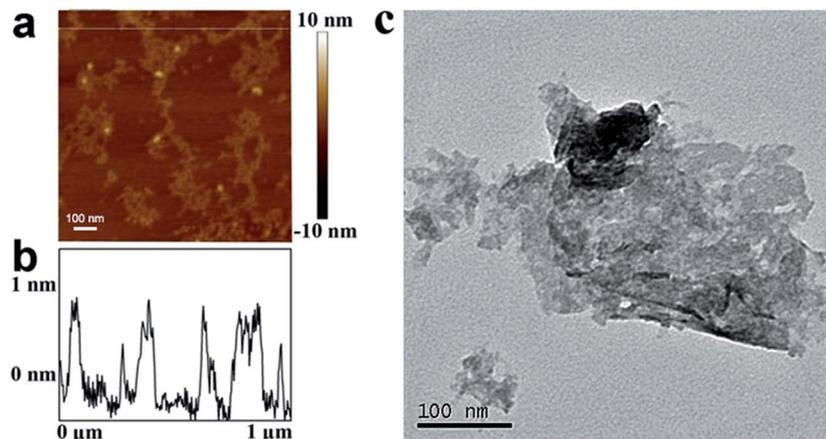
Fig. 1 (a) Atomic force microscopy images of the WS<sub>2</sub> nanosheets deposited on silica substrate, (b) the height profile diagram along the line labelled in (a). (c) Transmission electron microscopy image of one WS<sub>2</sub> nanosheet.
