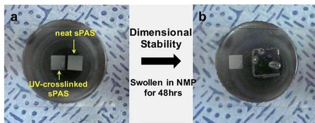
Fig. 5 Dimensional stability test of UV-crosslinked sPAS. (a) Two  $5 \times 5$  mm<sup>2</sup> size UV-crosslinked membranes were prepared. (b) The right-side membrane was swollen in NMP for 48 h.
