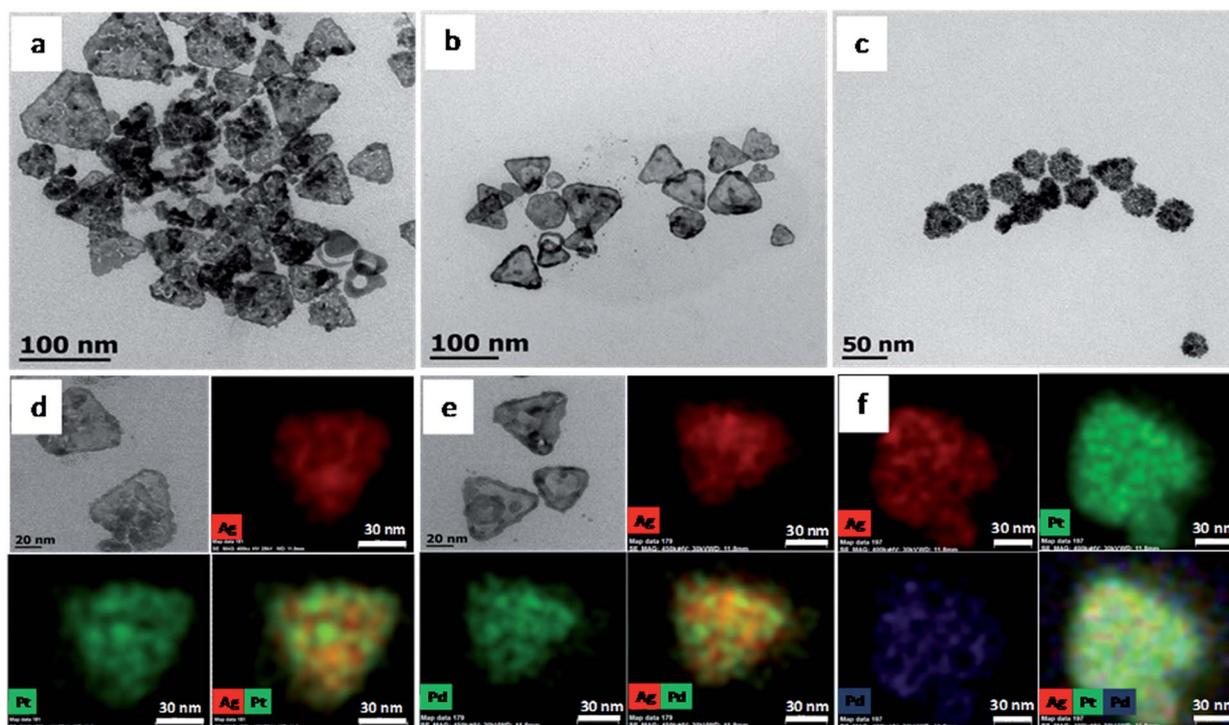
Fig. 2 TEM and STEM-EDX mapping images for (a and d) Ag@Pt, (b and e) Ag@Pd, and (c and f) Ag@PdPt nanoplates, respectively, prepared using the same procedure, except for the different metal precursors.
