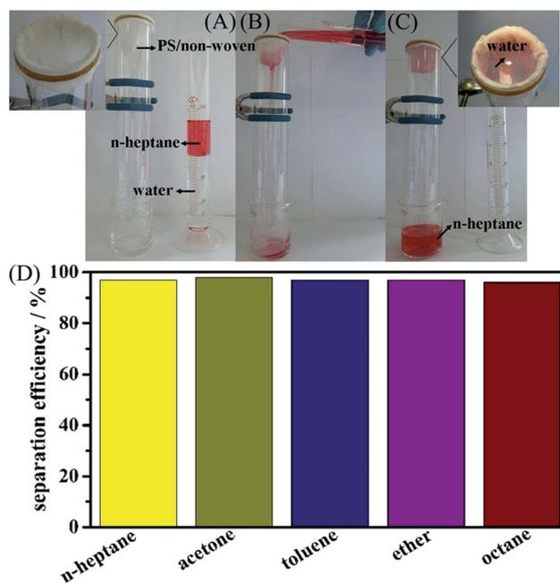
Fig. 10 (A–C) Optical images of the light oil *n*-heptane separation from *n*-heptane/water mixture (*n*-heptane colored with Sudan Red). (D) The separation efficiency of *n*-heptane, acetone, toluene, ether and octane from oil/water mixtures by using PS/non-woven fabric hybrid membranes.
