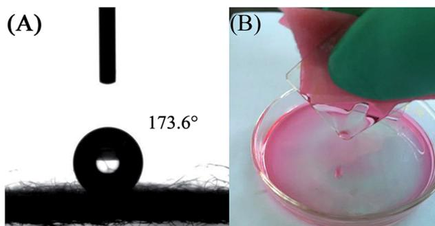
Fig. 4 (A) Photograph of a water droplet on PS/non-woven fabric hybrid membrane with a CA of  $173.6^\circ$ . (B) Optical image of chloroform (colored with Rhodamine B) adsorption for PS/non-woven fabric hybrid membrane.
