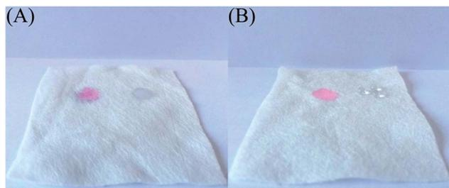
Fig. 3 Optical images of an oil droplet (left, 20  $\mu\text{L}$  chloroform colored with Rhodamine B) and water droplet (right, 20  $\mu\text{L}$  deionized water) on a non-woven fabric before (A) and after (B) modification by PS.
