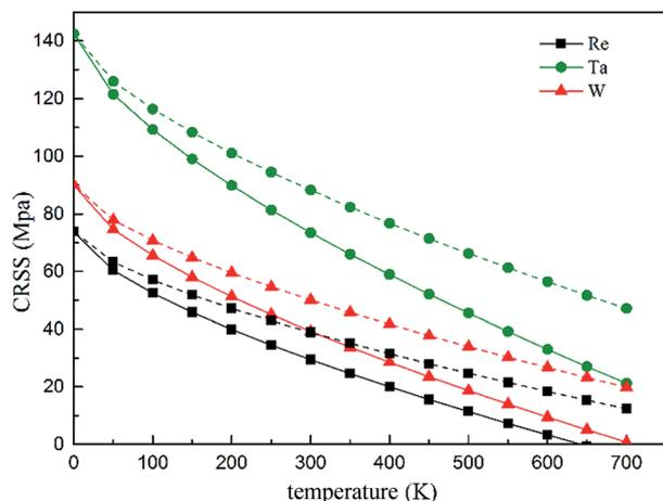
Fig. 14 Temperature and strain rate dependence of CRSS under the strain rate of  $6.67 \times 10^{-5} \text{ s}^{-1}$  (solid line) and  $2 \times 10^{-2} \text{ s}^{-1}$  (dashed line), respectively.
