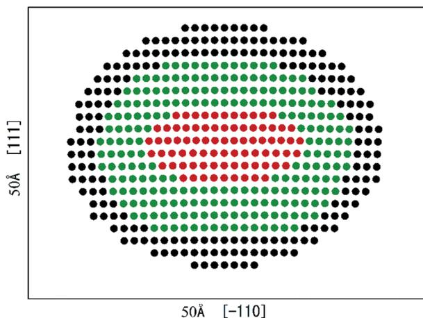
Fig. 2 Edge dislocation core equilibrium geometry in  $\gamma$  phase, separated into regions I (red atoms: dislocation core region), II (green atoms: bridging region) and III (black atoms: continuum region). The simulation cell is  $50 \text{ \AA} \times 50 \text{ \AA} \times 4.311 \text{ \AA}$  containing 495 atoms.
