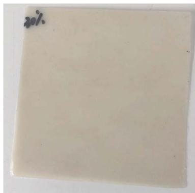
Fig. 3 Representative 7 : 3 m-HDPE : TPS composite.
