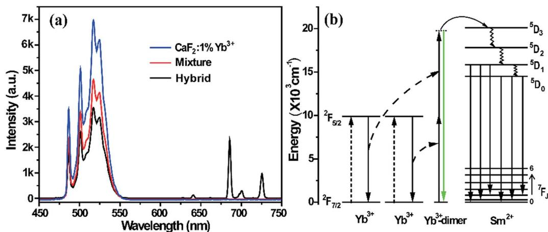
Fig. 2 (a) Emission spectra (450–750 nm) of the hybrid, CaF<sub>2</sub>:1%Yb<sup>3+</sup> and mixture materials upon 978 nm excitation at room temperature. (b) Schematic for the energy level diagram of Yb<sup>3+</sup> and Sm<sup>2+</sup> ions and possible UC population and emission processes.
