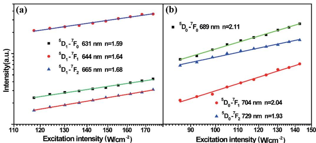
Fig. 4 (a) Excitation power dependence of the UCL of  ${}^5\text{D}_1 \rightarrow {}^7\text{F}_j$  ( $j = 0, 1, 2$ ) in  $\text{Sm}^{2+}$  ions. (b) Excitation power dependence of UCL of  ${}^5\text{D}_0 \rightarrow {}^7\text{F}_j$  ( $j = 0, 1, 2$ ) in  $\text{Sm}^{2+}$  ions.
