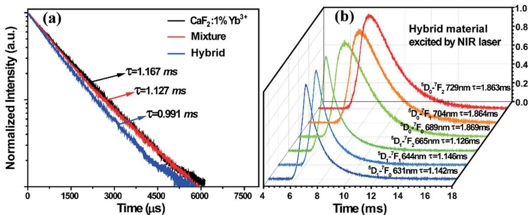
Fig. 3 (a) Decay curves of cooperative luminescence from  $\text{Yb}^{3+}$ -dimers by monitoring the 500 nm emission of  $\text{BaFCl}_{0.5}\text{Br}_{0.5}:1\%\text{Sm}^{2+}-\text{CaF}_2:1\%\text{Yb}^{3+}$ ,  $\text{CaF}_2:1\%\text{Yb}^{3+}$  and the mixture under 978 nm excitation. (b) UC photoluminescence decay curves of the  ${}^5\text{D}_j \rightarrow {}^7\text{F}_j$  transitions of  $\text{Sm}^{2+}$  ions at room temperature.
