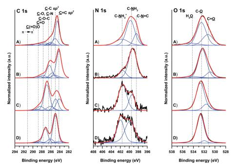
Fig. 1 High-resolution core-level C 1s, N 1s and O 1s XPS spectra of GO-NH<sub>2</sub> ((A) GO-1 and (B) GO-2) and GO ((C) GO-3 and (D) GO-4). The measured spectra are presented with black lines, while their corresponding fitted envelopes are presented in red. The individual contributions of different functional groups present in the materials are represented with blue lines.
