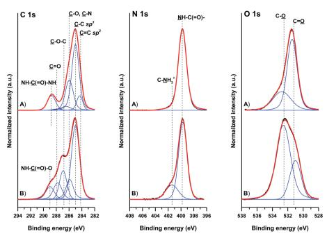
Fig. 4 High-resolution C 1s, N 1s and O 1s XPS spectra of (A) GO-NH<sub>2</sub> and (B) GO reacted with HDI. The measured spectra are presented with black lines, while their corresponding fitted envelopes are presented in red. The individual contributions of different functional groups present in the GO materials are represented with blue lines.
