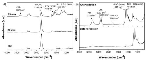
Fig. 2 (A) ATR-FTIR spectra of pure HDI and reaction mixtures after 20 and 95 min of reaction between GO-NH<sub>2</sub> and HDI in n-butyl acetate. (B) ATR-FTIR spectra of dried and washed GO-NH<sub>2</sub> before and after reaction with HDI.
