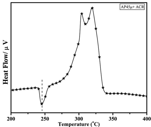
Fig. 11 DTA curve of AP<sub>45μ</sub> modified with industrial ACR (Cu–Cr–O).
