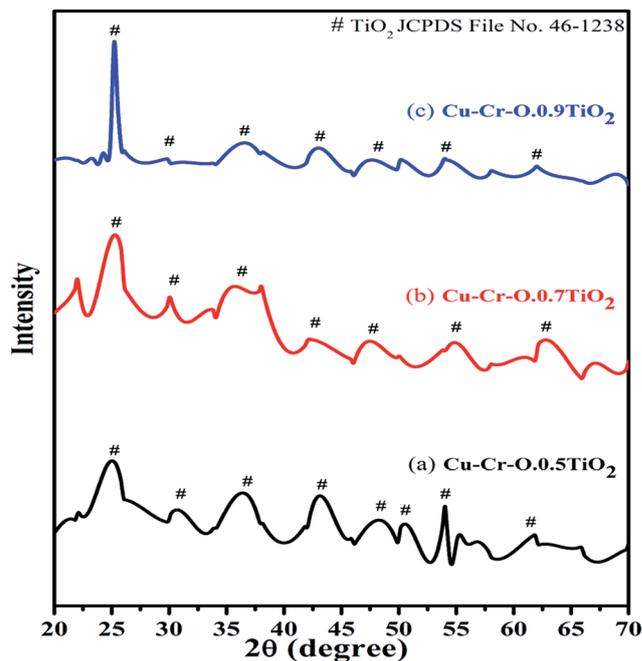
Fig. 2 XRD patterns of (a) Cu–Cr–O·0.5TiO<sub>2</sub>, (b) Cu–Cr–O·0.7TiO<sub>2</sub> and (c) Cu–Cr–O·0.9TiO<sub>2</sub> catalysts calcined at  $300^\circ \text{C}$ .
