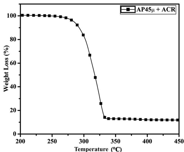
Fig. 12 TGA curve of AP<sub>45μ</sub> modified with industrial ACR (Cu–Cr–O).
