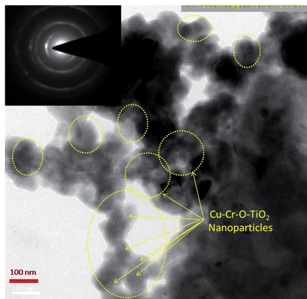
Fig. 8 TEM image of Cu-Cr-O·0.7TiO<sub>2</sub> calcined at 300 °C; the selected area electron diffraction (SAED) pattern is shown in the inset image.
