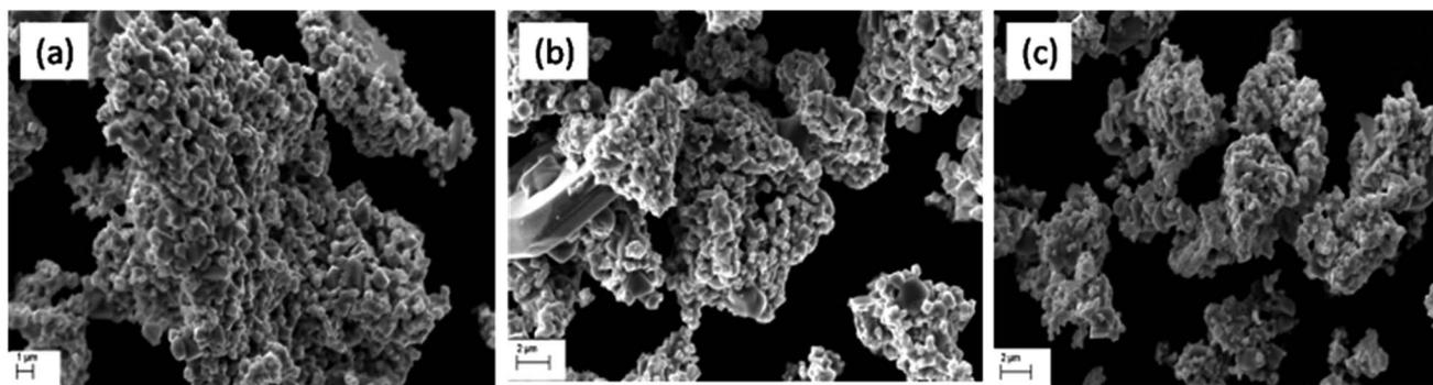
Fig. 6 SEM images of (a) Cu-Cr-O·0.5TiO<sub>2</sub>, (b) Cu-Cr-O·0.7TiO<sub>2</sub> and (c) Cu-Cr-O·0.9TiO<sub>2</sub> calcined at 300 °C.
