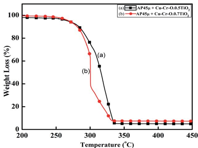
Fig. 14 TGA curves of AP<sub>45μ</sub> modified with (a) Cu–Cr–O–0.5TiO<sub>2</sub> and (b) Cu–Cr–O–0.7TiO<sub>2</sub> calcined at 300 °C.
