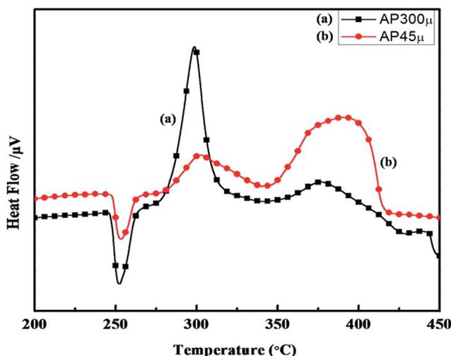
Fig. 9 DTA curves of (a) AP<sub>300μ</sub> and (b) AP<sub>45μ</sub>.
