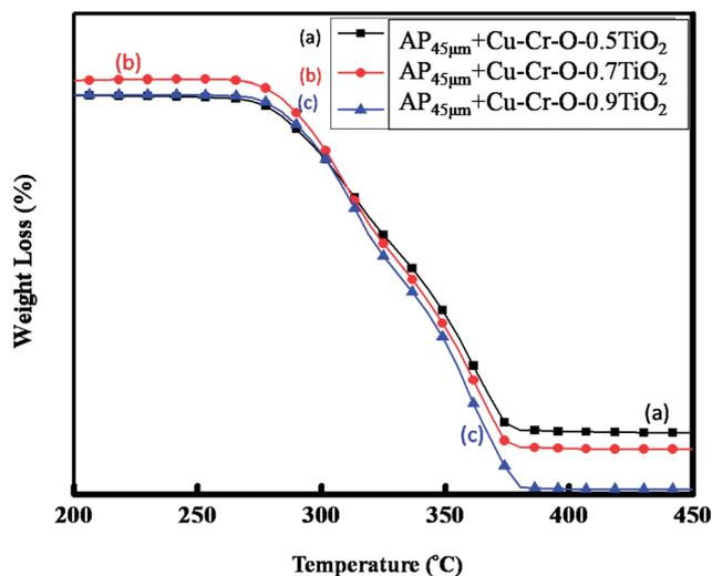
Fig. 16 TGA curves of AP<sub>45µm</sub> modified with (a) Cu–Cr–O·0.5TiO<sub>2</sub>, (b) Cu–Cr–O·0.7TiO<sub>2</sub> and (c) Cu–Cr–O·0.9TiO<sub>2</sub> calcined at 1050 °C.
