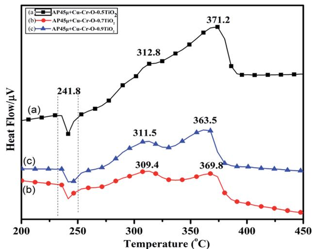
Fig. 15 DTA curves of AP<sub>45µm</sub> modified with (a) Cu–Cr–O·0.5TiO<sub>2</sub>, (b) Cu–Cr–O·0.7TiO<sub>2</sub> and (c) Cu–Cr–O·0.9TiO<sub>2</sub> calcined at 1050 °C.
