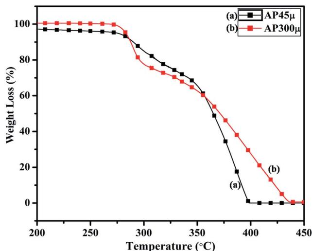
Fig. 10 TGA curves of (a) AP<sub>45μ</sub> and (b) AP<sub>300μ</sub>.
