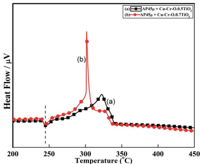
Fig. 13 DTA curves of AP<sub>45μ</sub> modified with (a) Cu–Cr–O–0.5TiO<sub>2</sub> and (b) Cu–Cr–O–0.7TiO<sub>2</sub> calcined at 300 °C.
