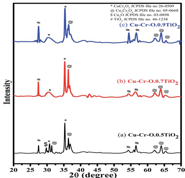
Fig. 3 XRD patterns of (a) Cu–Cr–O·0.5TiO<sub>2</sub>, (b) Cu–Cr–O·0.7TiO<sub>2</sub> and (c) Cu–Cr–O·0.9TiO<sub>2</sub> catalysts calcined at  $1050^\circ \text{C}$ .
