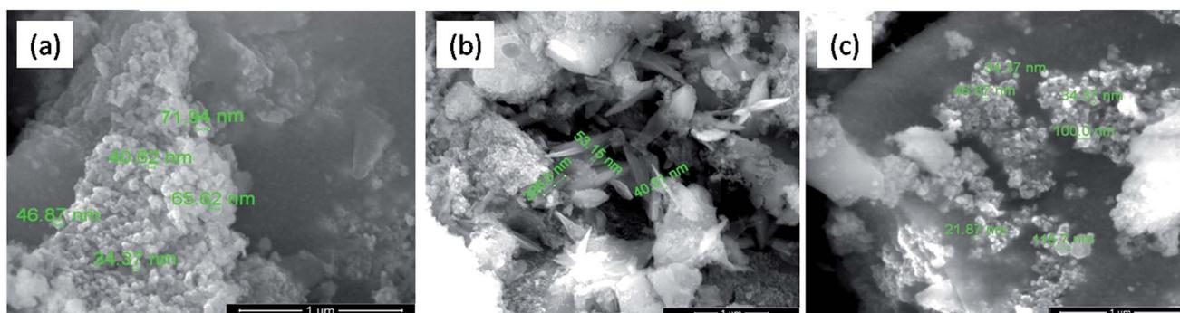
Fig. 7 SEM images of (a) Cu-Cr-O·0.5TiO<sub>2</sub>, (b) Cu-Cr-O·0.7TiO<sub>2</sub> and (c) Cu-Cr-O·0.9TiO<sub>2</sub> calcined at 1050 °C.
