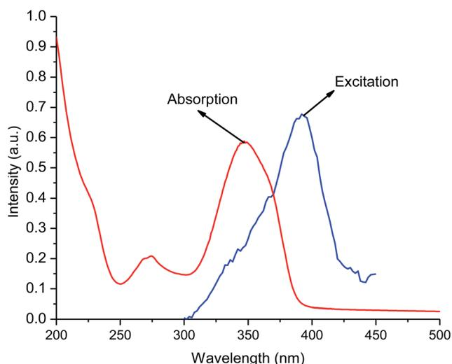
Fig. 6 Excitation and absorption spectra of the complex.
