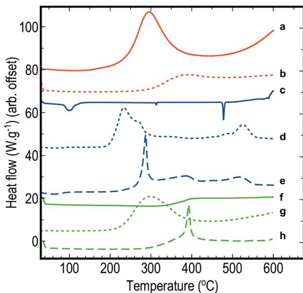
**Fig. 1** DSC scans of (a) blank pSi in air, (b) blank pSi in N<sub>2</sub>, (c) blank SP in air, (d) pSi/SP EM in air, (e) pSi/SP EM in N<sub>2</sub>, (f) blank PFPE in air, (g) pSi/PFPE EM in air, and (h) pSi/PFPE in N<sub>2</sub>.
