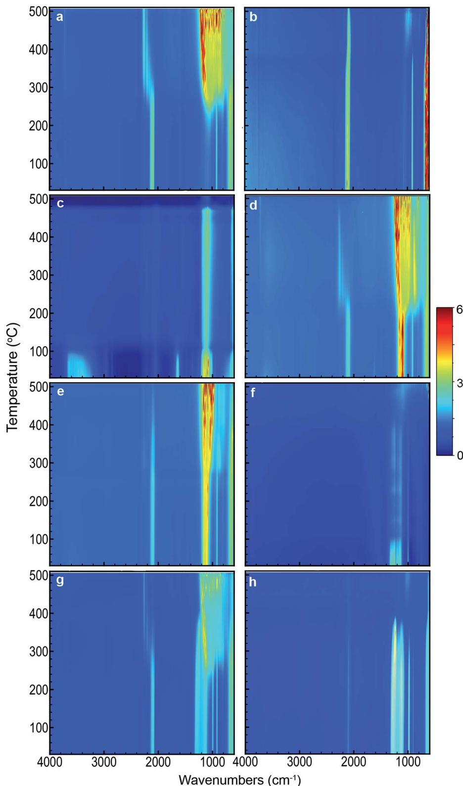
Fig. 2 2D FTIR spectra as a function of temperature of (a) blank pSi in air, (b) blank pSi in N<sub>2</sub>, (c) blank SP in air, (d) pSi/SP EM in air, (e) pSi/SP EM in N<sub>2</sub>, (f) blank PFPE in air, (g) pSi/PFPE EM in air, and (h) pSi/PFPE in N<sub>2</sub>.
