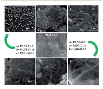
Fig. 26 FESEM images of bulk-polyaniline (PANI) (prepared without swollen liquid crystals (SLCs)) and nanostructured-PANI samples M= mixed, D= diffusion conditions, 5, 10, 20 is the aniline/cyclohexane (volume/volume ratio) in oil phase of swollen liquid crystals (SLCs).77 Reproduced with permission from Wiley-VCH.
