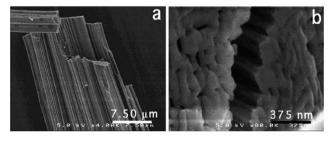
Fig. 23 SEM images of Zr needles (a) and close view of cross section (b). Reprinted with permission from ref. 78. Copyright 2004 American Chemical Society.
