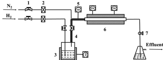
Fig. 2 Schematic diagram of oxidation device: (1) needle valve; (2) gas flowmeter; (3) heating jacket; (4) heating band; (5) temperature controller; (6) reaction chamber; (7) ball valve.
