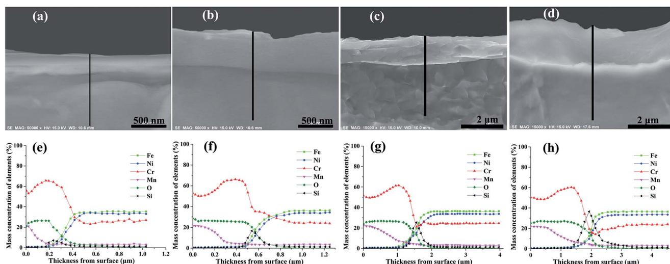
Fig. 4 Morphology and elemental distribution of the cross-section of oxide scales formed under  $H_2-H_2O$  environment after various isothermal oxidation times: (a, e) 0.2 h; (b, f) 2 h; (c, g) 10 h; (d, h) 20 h.
