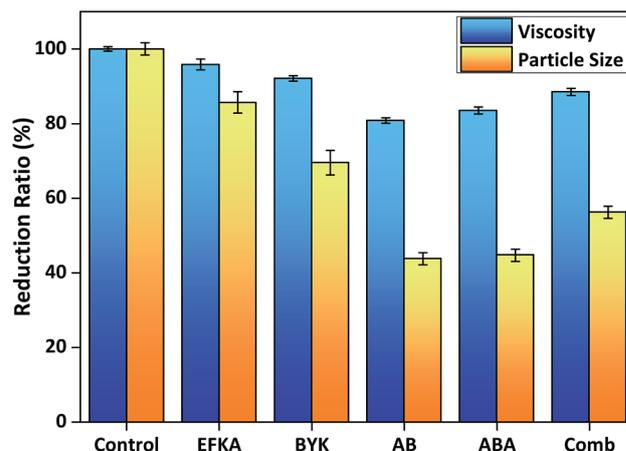
Fig. 5 Dispersion performance comparison between AB diblock, ABA triblock, comb and commercial polymeric dispersants (EFKA: EFKA-4310; BYK: BYK-2008; AB: PD30-*b*-PE40; ABA: PD30-*b*-PE60-*b*-PD30; comb: P(D30-co-PPGA15)).
