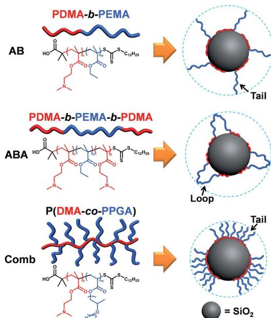
Scheme 1 Schematic representation of SiO<sub>2</sub> particle dispersion by AB diblock, ABA triblock and comb copolymer dispersants.
