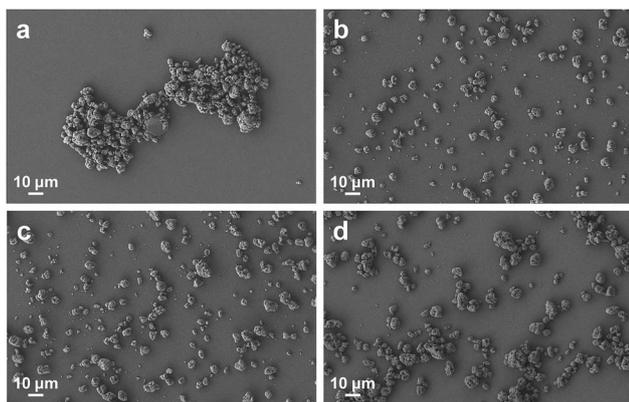
Fig. 6 SEM images of dispersed SiO<sub>2</sub> particles in xylene: (a) control sample without dispersant; (b) AB diblock: PD30-*b*-PE40; (c) ABA triblock: PD30-*b*-PE60-*b*-PD30; (d) comb: P(D30-*co*-PPGA15).
