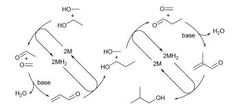
Scheme 3 Co-condensation of MeOH and EtOH via a hydrogen borrowing mechanism.
