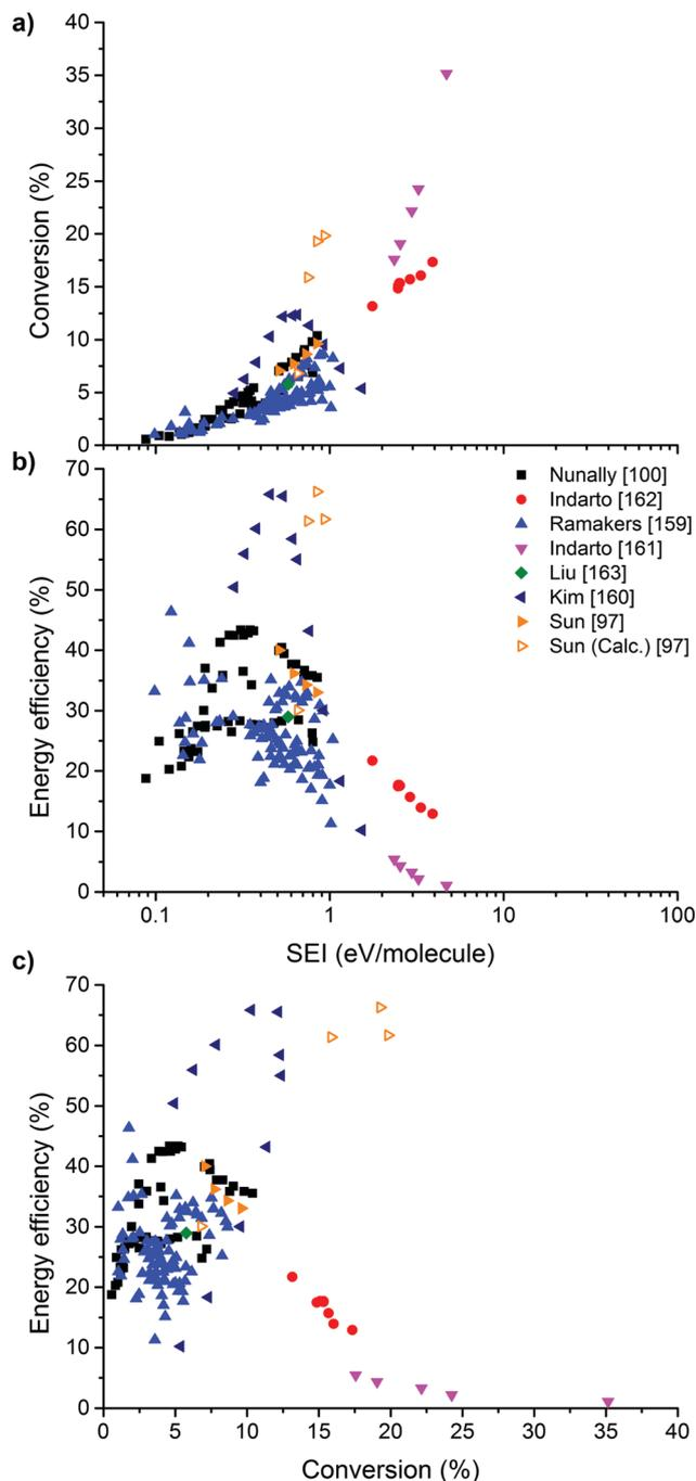
Fig. 22 Experimental data collected from the literature for  $\text{CO}_2$  splitting in a GA, showing the conversion (a) and energy efficiency (b) as a function of the SEI, as well as the energy efficiency as a function of the conversion (c). Note that some of the data have been recalculated from the original references to take, among others, dilution effects into account.
