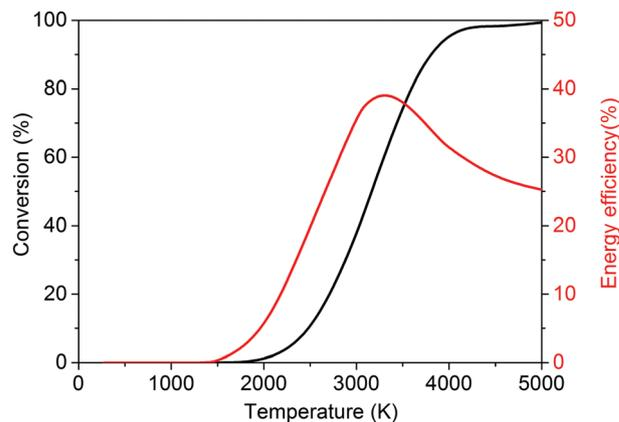
Fig. 4 Calculated theoretical thermal conversion (left axis) and corresponding energy efficiency (right axis) as a function of temperature for the conversion of CO<sub>2</sub> and H<sub>2</sub>O into H<sub>2</sub>, CO and O<sub>2</sub>.
