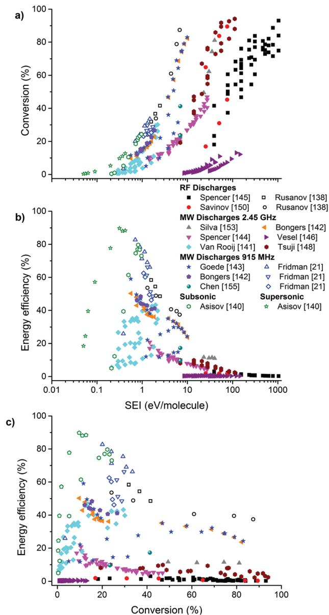
Fig. 21 Experimental data collected from the literature for CO<sub>2</sub> splitting in MW and RF discharges, showing the conversion (a) and energy efficiency (b) as a function of the SEI, as well as the energy efficiency as a function of the conversion (c). The open symbols represent the data from the 1970–1980s. Note, some of the data have been recalculated from the original references to take, among others, dilution effects into account.
