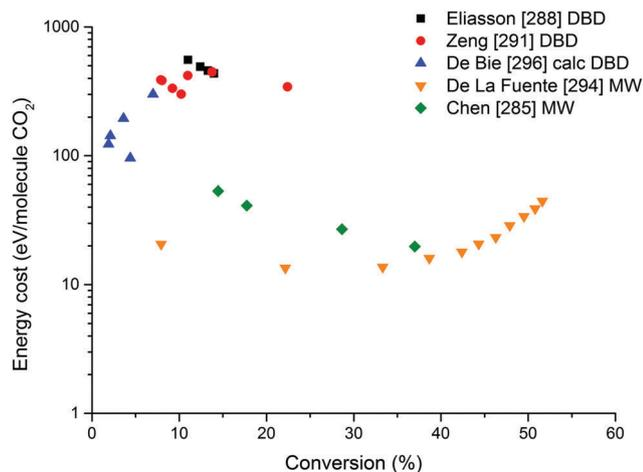
Fig. 34 Comparison of all the data collected from the literature for CO<sub>2</sub> hydrogenation in the different plasma types, showing the energy cost per converted CO<sub>2</sub> molecule as a function of the conversion. Note, some of the data have been recalculated from the original references to take, among others, dilution effects into account.
