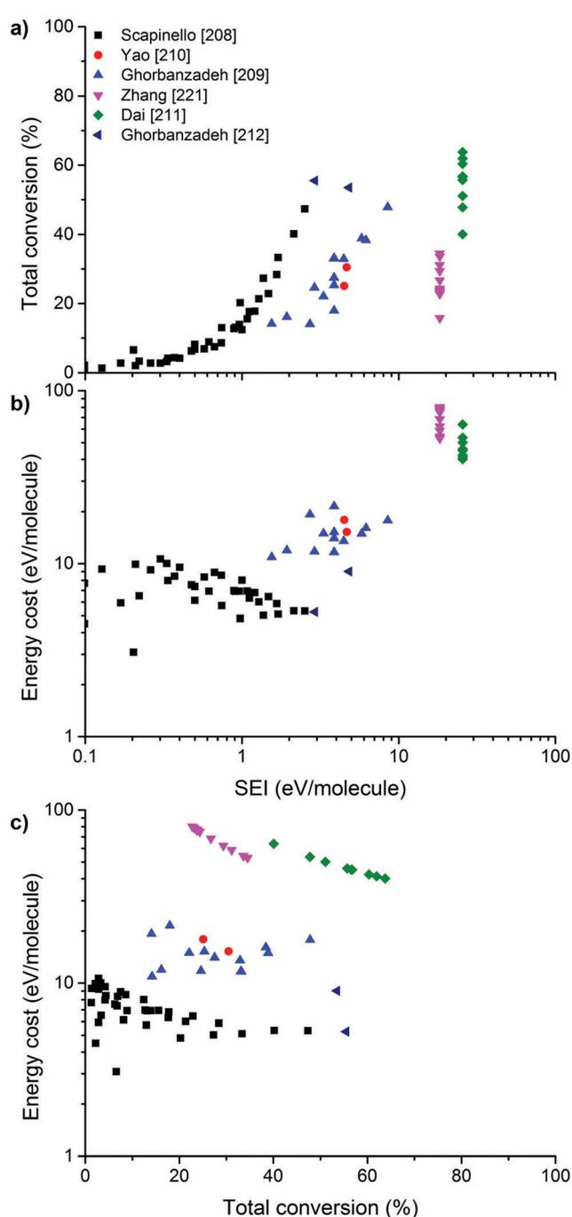
**Fig. 31** Experimental data collected from the literature for DRM in nanosecond pulsed discharges, showing the conversion (a) and energy cost (b) as a function of the SEI, as well as the energy cost as a function of the conversion (c). Note that some of the data have been recalculated from the original references to take, among others, dilution effects into account.
