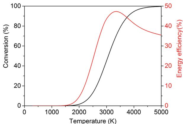
Fig. 2 Calculated theoretical thermal conversion (left axis) and corresponding energy efficiency (right axis) as a function of temperature for the pure splitting of  $\text{CO}_2$  into  $\text{CO}$  and  $\text{O}_2$ .
