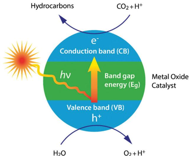
Fig. 7 Principle of the photochemical reduction of CO<sub>2</sub> by water on a photocatalyst.
