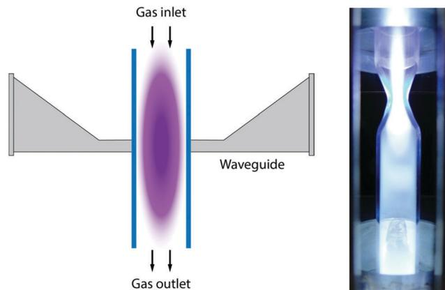
Fig. 14 Schematic (left) and image (right; courtesy of Dutch Institute For Fundamental Energy Research (DIFFER)) of a MW discharge.
