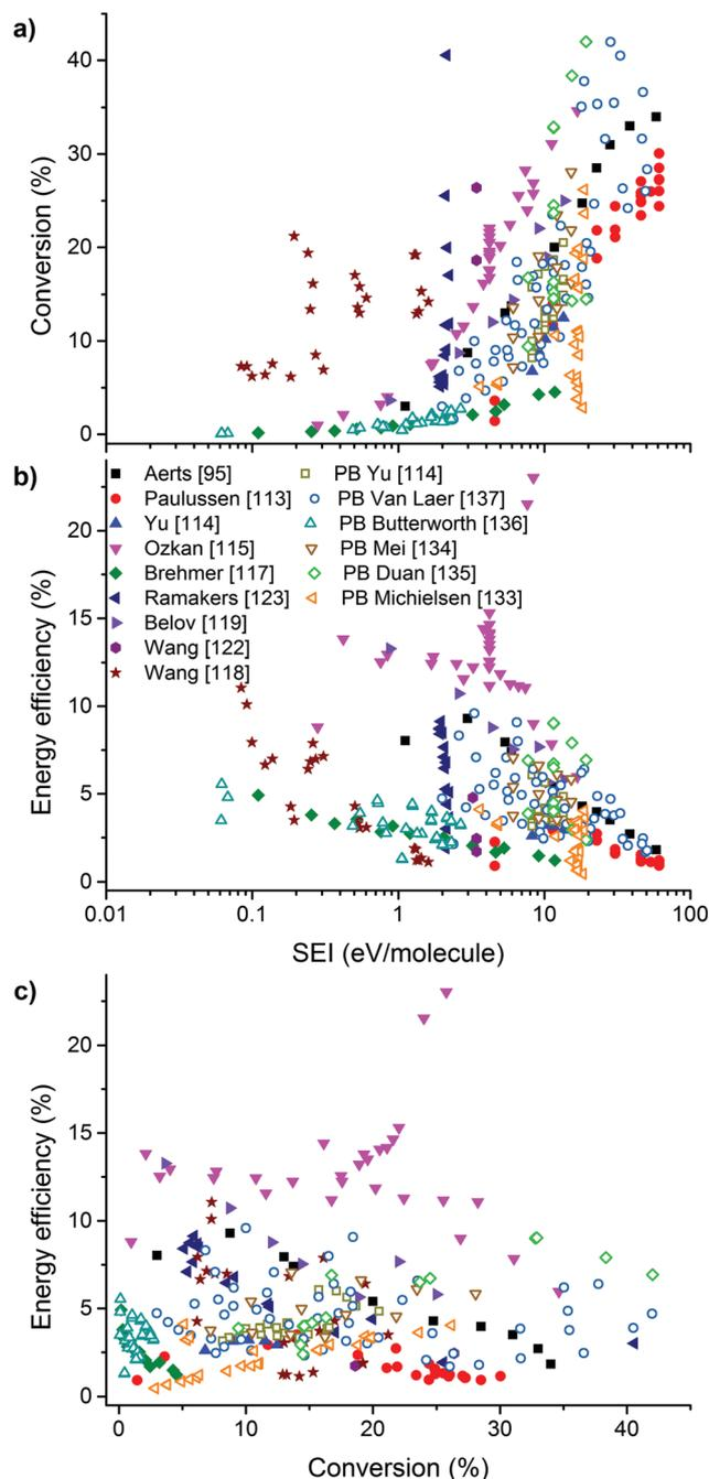
Fig. 20 Experimental data collected from the literature for CO<sub>2</sub> splitting in a DBD, showing the conversion (a) and energy efficiency (b) as a function of the SEI, as well as the energy efficiency as a function of the conversion (c). The open symbols represent the data with a packed bed (PB). Note, some of the data have been recalculated from the original references to take, among others, dilution effects into account.
