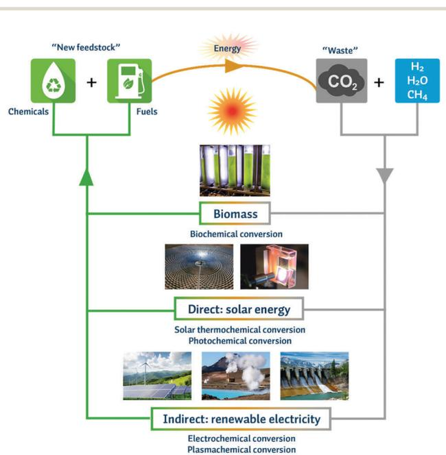
Fig. 1 Overview of the different novel technologies and their principal use of renewable energy for the conversion of CO<sub>2</sub> in a carbon neutral cycle.
