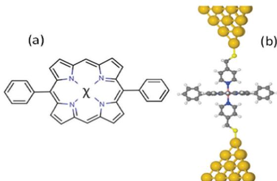
Fig. 1 Diphenylporphyrins-based molecular structures (a) with metallic atom, (b) an example of an optimized configuration of the system containing a single molecule  $\chi$ -DPP sandwiched between two gold leads which in turn are activated by pyridine-4-yl-methanethiol with different metallic atoms, where  $\chi = \text{Co}, \text{Cu}, \text{Ni}$  or  $\text{Zn}$ .
