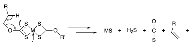
Scheme 1 A generalised breakdown mechanism proposal for the xanthate precursors. M = Ca, Ba or Cu, L = i PrOH or PPh 3 , R = i Pr or 2-methoxyethyl.
