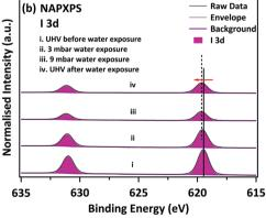
Fig. 1 NAPXPS spectra of (a) Pb 4f & Sr 3d, and (b) I 3d core levels under various conditions as noted (before/during/after water exposure). All the spectra are normalised to the corresponding integrated area of the Sr 3d<sub>5/2</sub>
