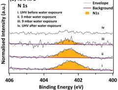
Fig. 2 NAPXPS spectra of (a) C 1s & Sr 3p, and (b) N 1s core levels before/during/after water exposure. All spectra are normalised to the corresponding integrated area of the Sr  $3d_{5/2}$  peak.
