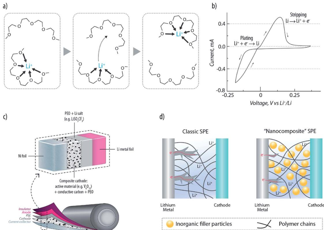
Fig. 2 (a) Schematic drawing of Li<sup>+</sup> transport in a PEO matrix, assisted by the segmental motion of the polymeric chains.<sup>18</sup> (b) Cyclic voltammetry showing the reversible Li stripping–plating achievable with a PEO-based PSE. (c) Example of a typical lithium-polymer battery (LPB) configuration. (d) Schematic representation of dendrite growth suppressed by the nanocomposite SPE.<sup>36</sup>
