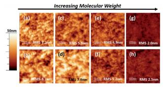
Fig. 3 AFM images with indicated RMS values for PTB7: $C_{71}$ -PCBM blends before (a, c, e, g) and after (b, d, f, h) light soaking. (a, b) PTB7-1: $C_{71}$ -PCBM; (c, d) PTB7-2: $C_{71}$ -PCBM; (e, f) PTB7-3: $C_{71}$ -PCBM; (g, h) PTB7-4: $C_{71}$ -PCBM.
