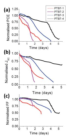
Fig. 4 Device characteristics for non-encapsulated PTB7-1-4:C<sub>71</sub>-PCBM inverted solar cells as a function of time under illumination of 1 sun. Each parameter was normalised to the initial value at the start of the aging process.
