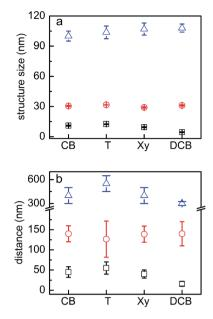
Fig. 6 Characteristic structure sizes (a) and distances (b) of P3HT:PCBM films post-treated with chlorobenzene, toluene, xylene and dichlorobenzene vapors. The values are obtained from the fitting parameters of the horizontal line cuts of 2D GISAXS data.
