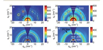
Fig. 8 2D GIWAXS data of P3HT:PCBM films post-treated with chlorobenzene (a), toluene (b), xylene (c) and dichlorobenzene (d) vapors. Dominant PCBM Bragg peak 1, peak 2 and peak 3 are marked as black, yellow and red circles in (a) and (b), respectively
