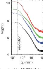
Fig. 5 Horizontal line cuts of the 2D GISAXS data of P3HT:PCBM films post-treated using chlorobenzene (black), toluene (blue), xylene (green) and dichlorobenzene (red) vapors. Solid lines (grey) are the fits as explained in the text. The curves are shifted along the intensity axis for clarity. The dashed line represents the resolution limit to larger structures.
