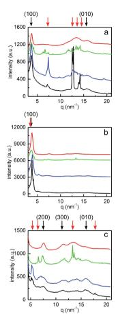
Fig. 9 Horizontal (a) and vertical (b) sector integrals performed on 2D GIWAXS data of P3HT:PCBM films post-treated with chlorobenzene (black), toluene (blue), xylene (green) and dichlorobenzene (red) vapors. Vertical sector integrals above 5 nm<sup>-1</sup> are shown in (c). The black and red arrows denote the scattering signal from P3HT and PCBM crystallites, respectively. The curves are shifted along the intensity axis for clarity.
