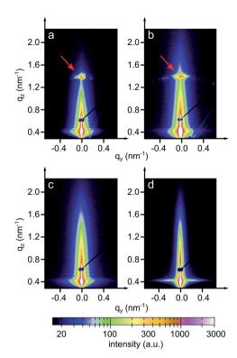
Fig. 4 2D GISAXS data of P3HT:PCBM films post-treated with chlorobenzene (a), toluene (b), xylene (c) and dichlorobenzene (d) vapors, respectively. The Bragg peaks are marked with red arrows. The specular peak is shielded with a point-shaped beamstop
