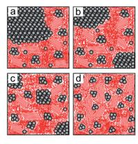
Fig. 10 Schematic morphology of P3HT:PCBM films post-treated with chlorobenzene (a), toluene (b), xylene (c) and dichlorobenzene (d) vapors. The grey spheres correspond to PCBM, red tangled lines represent amorphous P3HT and red parallel lines are related to P3HT crystallites
