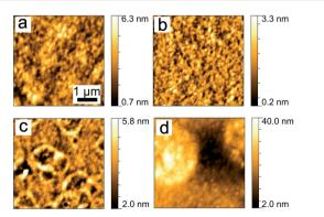
Fig. 3 AFM images  $(4 \times 4) \mu m^2$  of P3HT:PCBM films, post-treated with chlorobenzene (a), toluene (b), xylene (c) and dichlorobenzene (d) vapors. The corresponding rms roughness values are 8.6 Å, 4.7 Å, 7.8 Å and 79.8 Å, respectively.
