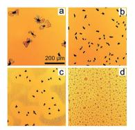
Fig. 2 Optical microscopy images of P3HT:PCBM films post-treated with chlorobenzene (a), toluene (b), xylene (c) and dichlorobenzene (d) vapors. All images have an identical size.
