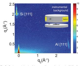
**Fig. 2** Background signals of the pure silicon wafer show the [111] reflection normal to the wafer. The aluminum[111] reflection is observed in the plane of the wafers as contribution from the sample can.
