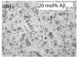
Fig. 3 Optical microcopy images of a (a) pure POPC/DMPS membrane and (b) a POPC/DMPS + 20 mol%  $A\beta_{25-35}$ . While the pure lipid matrix shows a smooth surface, inclusions were observed at peptide concentrations of 10 and 20 mol%.
