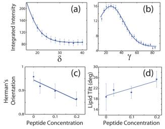
Fig. 9 (a) Intensity of the second reflectivity Bragg peak as a function of angle  $\delta$  from the  $q_z$  axis. (b) Integrated intensity of the lipid correlation peak as a function of angle  $\gamma$  from the  $q_{\parallel}$  axis. (c) Hermans orientation function, as defined in the Materials and methods section in eqn (1), for membrane bending for all peptide concentrations and (d) lipid tail tilt angle for all peptide concentrations.
