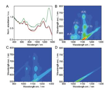
Fig. 7 (A) UV-vis-NIR absorption spectra of pristine (7,6)-enriched SWNTs (black), and the products of their reactions with 3 in TCE (red) and DMF (green). (B) PLE spectrum of pristine (7,6)-enriched SWNTs and the products of their reactions with 3 in TCE (C) and DMF (D). All spectra in  $D_2O$  with 1% sodium dodecylsulfate as surfactant and acquired at room temperature. Scattering has not been filtered.
