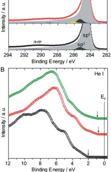
Fig. 8 (A) XPS spectra of C 1s core level for the pristine SWNTs (lower panel, black circles and line), functionalized with 3 in TCE (middle panel, red circles and line) and in DMF (upper panel, green circles and line). Circles are experimental data and the lines represent the fits. (B) UPS spectra measured with He I line of the pristine SWNTs (black circles), functionalized with 3 in TCE (red circles) and in DMF (green circles).
