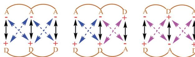
Fig. 1 Electrostatic interactions between H-bond acceptors and donors in triply H-bonded complexes as proposed by Jorgensen *et al.*; A and D symbolize hydrogen bond acceptor and donor atoms respectively; black, blue and pink arrows represent attractive primary, attractive secondary and repulsive secondary interactions, respectively; the association constant decreases with an increasing number of repulsive secondary interactions.
