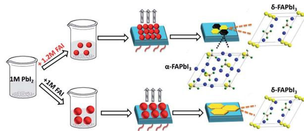
Fig. 5 Schematic view of the possible crystal growth process of FAPbI<sub>3</sub> films *via* controllable precursors. The unit cell of FAPbI<sub>3</sub>: yellow: Pb; gray: C; green: N; blue: I.
