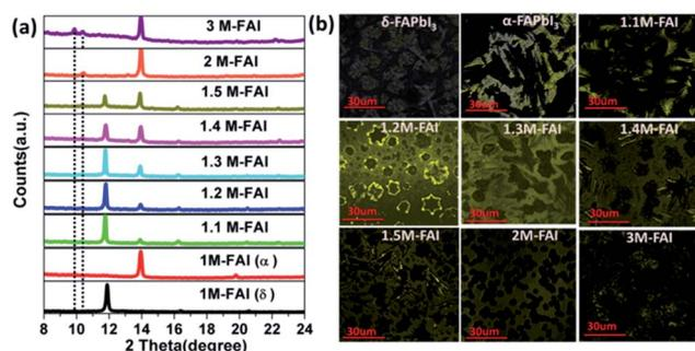
Fig. 1 XRD patterns (a) and confocal fluorescence microscopy images (b) of the FAPbI<sub>3</sub> films formed with different FAI/PbI<sub>2</sub> molar ratios from 1 to 3. All the films were annealed at low temperature (60 °C), except for pure  $\alpha$ -FAPbI<sub>3</sub> at 170 °C. For confocal fluorescence microscopy, all the films were excited at 485 nm, except for  $\delta$ -FAPbI<sub>3</sub> at 405 nm.
