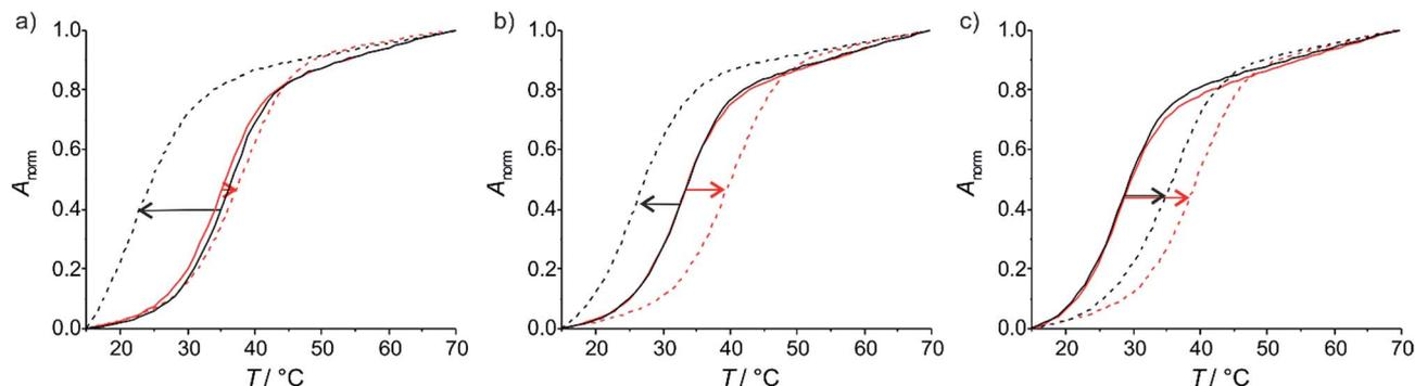
Fig. 2 Melting curves of the duplexes in the absence (solid lines) and presence (dotted lines) of one equivalent of  $\text{AgNO}_3$ . The red melting curves belong to the duplex comprising a cytosine residue opposite to P, the black ones to that with a thymine residue. (a) pH 5.5, (b) pH 6.8, (c) pH 9.0.
