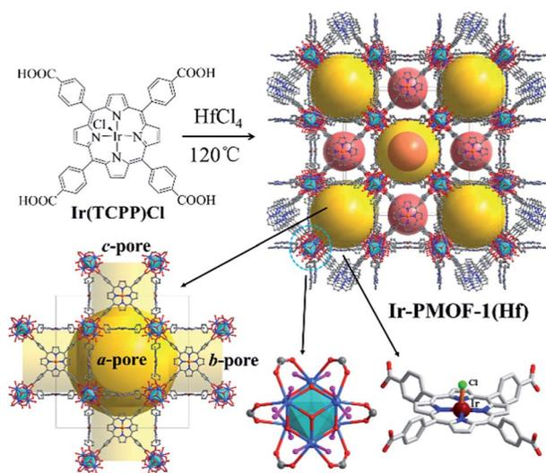
Fig. 1 Assembly of 3D Ir-PMOF-1(Hf) based on 6-connected Hf<sub>6</sub>(μ<sub>3</sub>-O)<sub>8</sub>(OH)<sub>2</sub>(H<sub>2</sub>O)<sub>10</sub> clusters and 4-connected Ir(TCPP)Cl ligands, showing two types of cavities interconnected to generate open channels in three directions.
