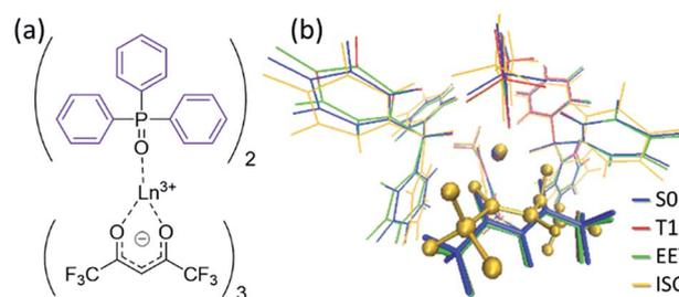
Fig. 3 (a) Chemical structure and (b) the optimized geometries of the  $\text{Tb}(\text{hfa})_3(\text{tppo})_2$  complex. Blue, red, green, and yellow in (b) are the LMs on  $\text{S}_0$ ,  $\text{T}_1$ , and the MSXs for the EET and ISC processes, respectively. Geometrical optimizations were carried out using the ONIOM( $\omega\text{B97XD}$ :UFF) method, in which the phenyl groups of tppo (purple in (a)) and others (black in (a)) were treated as the low- and high-level regions, respectively.
