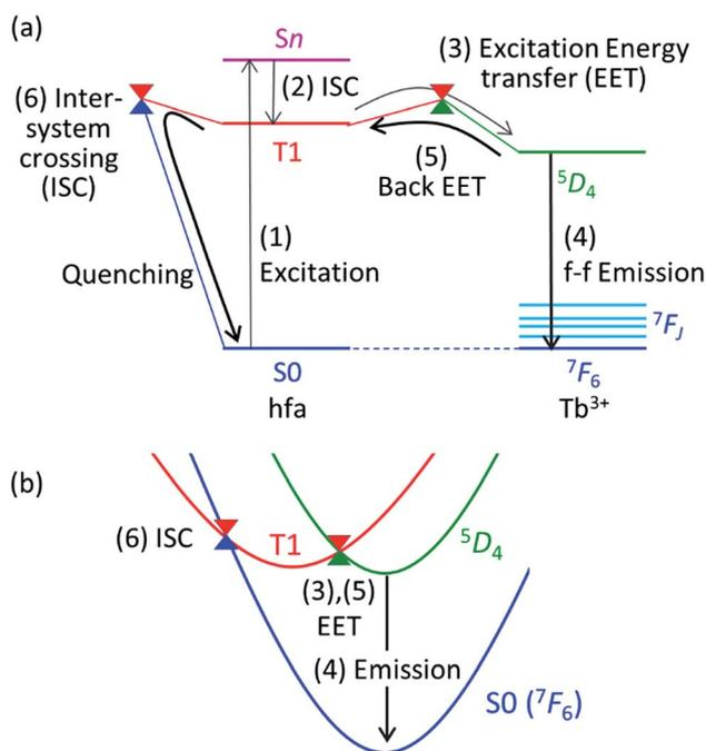
Fig. 2 Emission and quenching mechanisms of  $\text{Tb}^{3+}$  coordinated by hfa ligands shown in the Jablonski diagram (a) and the schematic potential energy surfaces (PESs) (b).  $S_n$  (or  $T_1$ ) and  $2^{5+1}L_J$  represent the electronic states of hfa and  $\text{Tb}^{3+}$ , respectively.
