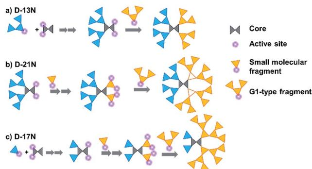
Fig. 2 “Converge-then-diverge” methods to construct Janus dendrimers.
