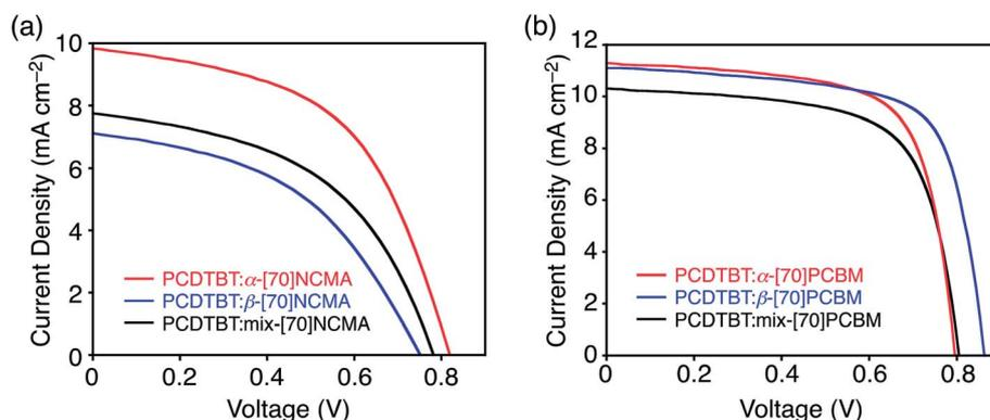
**Fig. 3** Current density–voltage curves averaged from ten independent PSC devices based on (a) PCDTBT :  $\alpha$ -[70]NCMA (red), PCDTBT :  $\beta$ -[70]NCMA (blue) and PCDTBT : mix-[70]NCMA (black), and (b) PCDTBT :  $\alpha$ -[70]PCBM (red), PCDTBT :  $\beta$ -[70]PCBM (blue) and PCDTBT : mix-[70]PCBM (black) films.
