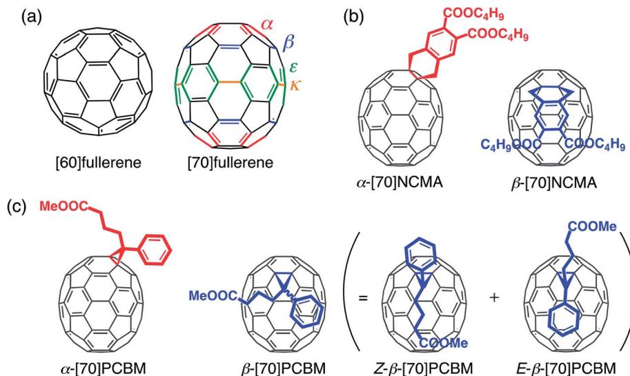
Fig. 1 (a) Structures of [60]fullerene and [70]fullerene;  $\alpha$ -,  $\beta$ -,  $\epsilon$ - and  $\kappa$ -type [6,6]-bonds of [70]fullerene are represented by red, blue, green and orange lines, respectively. (b) Structures of [70]NCMA isomers. (c) Structures of [70]PCBM isomers.
