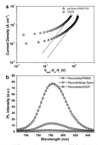
Fig. 4 (a) The space-charge-limited-current (SCLC) of hole-only devices with the configuration of indium tin oxide (ITO)/poly(3,4-ethylenedioxythiophene)-polystyrene sulfonate (PEDOT:PSS)/p,p-spiro-OMeTAD or IDIDF (with Li-bis(trifluoromethanesulfonyl)imide (Li-TFSI) and 4-tert-butylpyridine (tBP) as additives)/Au. (b) PL emission spectra of perovskite/PMMA, perovskite/p,p-spiro-OMeTAD, and perovskite/IDIDF film under excitation at 670 nm.
