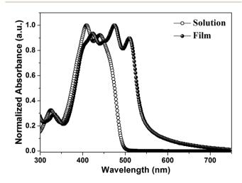
Fig. 2  $\,$  UV-vis absorption spectra of IDIDF in a solution (tetrahydrofuran,  $1\times 10^{-5}$  M) and film state.
