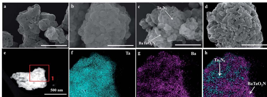
Fig. 2 FESEM images of typical samples: (a)  $\text{Ta}_3\text{N}_5$ , (b)  $\text{BaTaO}_2\text{N}$ , (c) a mixture of  $\text{Ta}_3\text{N}_5$  and  $\text{BaTaO}_2\text{N}$ , and (d)  $\text{Ba}(0.3)\text{-Ta}_3\text{N}_5$  (the scale bar is 500 nm). Elemental mappings of  $\text{Ba}(0.3)\text{-Ta}_3\text{N}_5$ : (e) TEM image, (f) Ta element, (g) Ba element, and (h) simulated dispersion of  $\text{Ta}_3\text{N}_5$  and  $\text{BaTaO}_2\text{N}$ .
