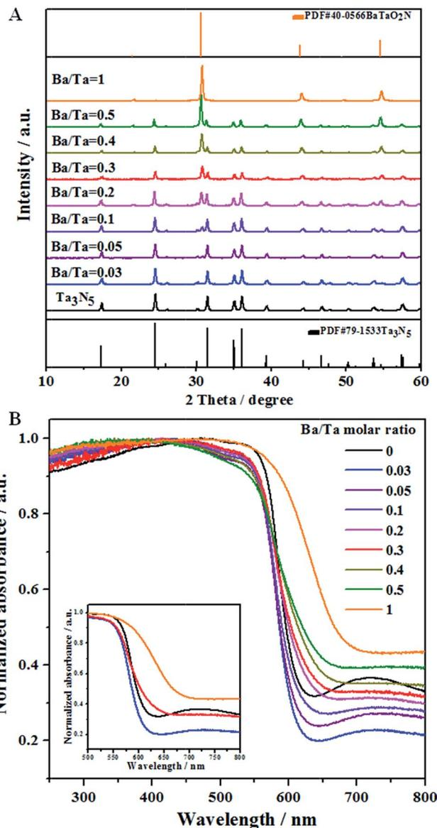
Fig. 1 Structural characterizations of typical Ba( $n$ )-Ta<sub>3</sub>N<sub>5</sub> samples ( $n = 0-1$ ): (A) XRD patterns and (B) UV-vis spectra. " $n$ " stands for the molar ratio of Ba/Ta. The inset figure is enlarged for the wavelength range of 500–800 nm.
