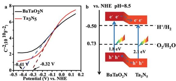
Fig. 4 Band structure characterizations of the  $Ta_3N_5$  and BaTaO<sub>2</sub>N samples. (a) Mott-Schottky plot for the  $Ta_3N_5$  and BaTaO<sub>2</sub>N electrodes. Electrolyte: 0.5 M Na<sub>2</sub>SO<sub>4</sub> solution (pH = 8.5, adjusted using NaOH). Frequency: 1000 Hz. (b) The relative band positions of the  $Ta_3N_5$ /BaTaO<sub>2</sub>N heterostructure.
