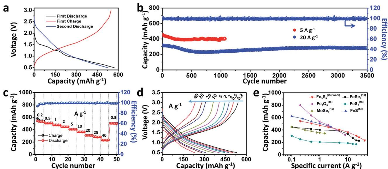
Fig. 2 Electrochemical performance of the as-prepared Fe<sub>3</sub>S<sub>4</sub>. (a) Discharge–charge curves of the first two cycles at a specific current of 0.2 A g<sup>-1</sup>; (b) cycling performances at 5 and 20 A g<sup>-1</sup>; (c) rate capability and (d) discharge–charge curves at various current rates; (e) comparison of the as-prepared Fe<sub>3</sub>S<sub>4</sub> with other conversion anode materials of SIBs.
