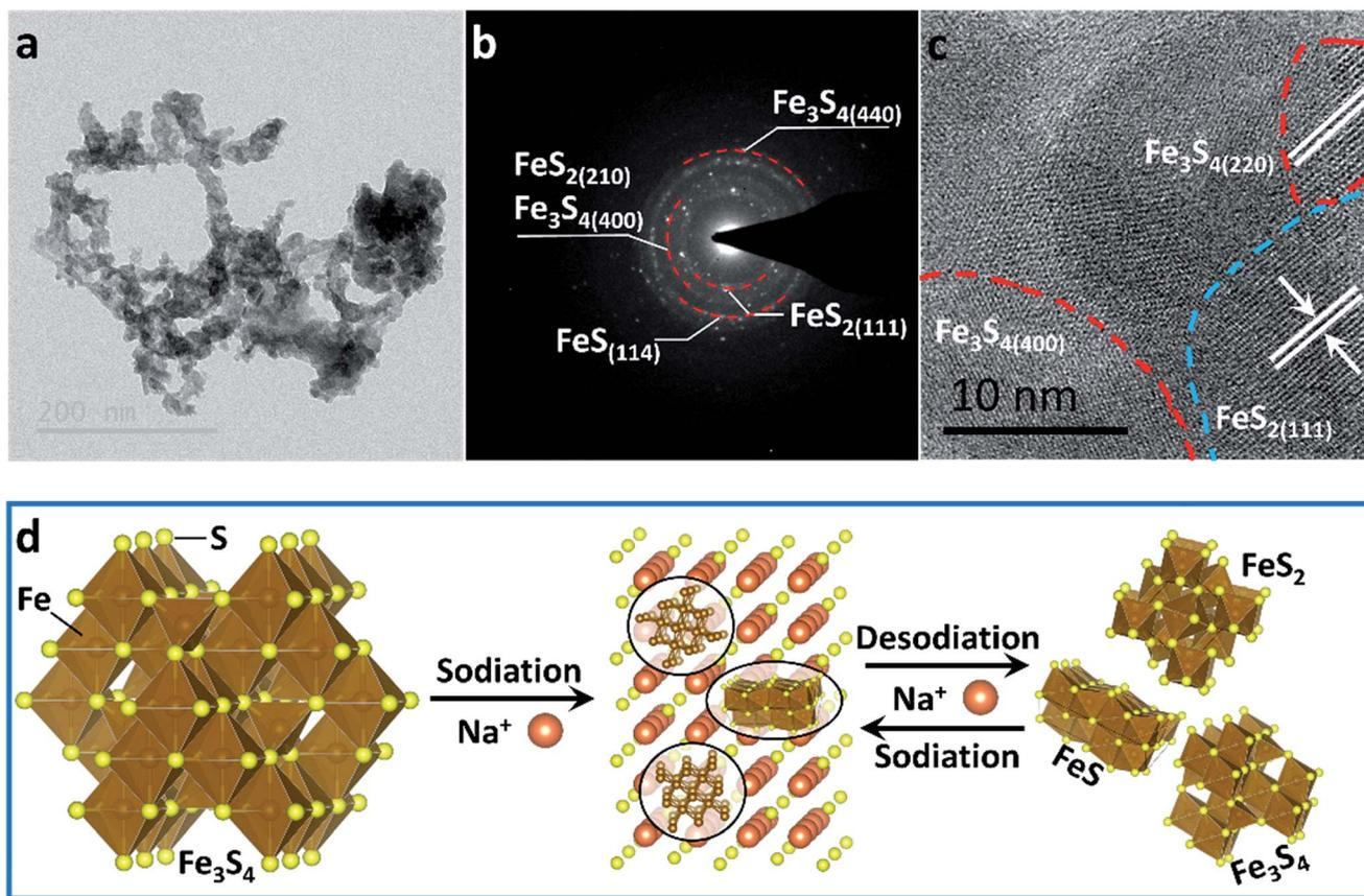
Fig. 4 (a) TEM image, (b) SAED pattern and (c) HRTEM image of the as-prepared  $\text{Fe}_3\text{S}_4$  at a full charge state after 200 cycles. (d) Schematic illustration of the sodium-storage mechanism in the  $\text{Fe}_3\text{S}_4$  electrode.
