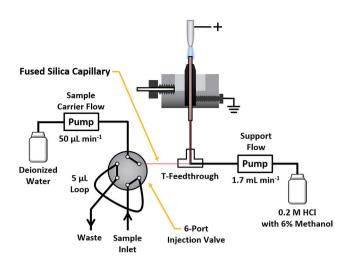
Fig. 1 Schematic of the SCGD design and flow-injection arrangement used to introduce peptide solutions into the discharge.
