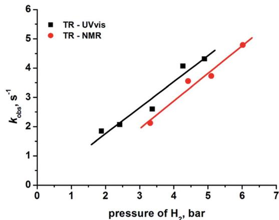
Fig. 4 Plots of pseudo-first-order rate constants  $k_{\text{obs}}$  determined from the decay of the transients obtained by TR-NMR (black squares) and TR-UV-vis (red circles) after 355 nm excitation of complex **2** in benzene vs. the pressure of quenching gas ( $\text{H}_2$ ). The corresponding lines of best fit are shown in black and red.
