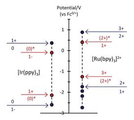
Fig. 5 Redox potentials for ground states (blue dots) and electronically excited states (red dots) within the  $[Ru(bpy)_3]^{2+}-[Ir(ppy)_3]$  mixed annihilation ECL system.
