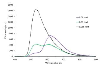
Fig. 3 Annihilation ECL spectra  $(0.99 \text{ V to } -2.77 \text{ V vs. } \text{Fc}^{0/+})$  for a mixture of [lr(ppy)<sub>3</sub>] (0.25 mM) and [Ru(bpy)<sub>3</sub>]<sup>2+</sup> (0.015-0.060 mM) in acetonitrile with 0.1 M [TBA][PF<sub>6</sub>]. For each spectrum, a two-step potential pulse was applied at 0.5 Hz for 12 s.
