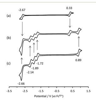
Fig. 1 Cyclic voltammograms of: (a)  $[Ir(ppy)_3]$ ; (b) a mixture of  $[Ir(ppy)_3]$ and  $[Ru(bpy)_3]^{2+}$ ; and (c)  $[Ru(bpy)_3]^{2+}$ , showing  $E^{\circ}$  values. All complexes at 0.25 mM with 0.1 M [TBA][PF $_6$ ] supporting electrolyte in acetonitrile. Scan rate: 0.1 V s<sup>-1</sup>
