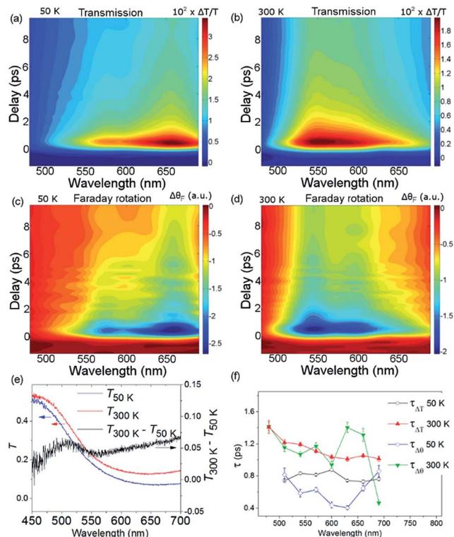
Fig. 3 Spectro-temporal dynamics of the transmission and magneto-optical Faraday response for  $T_s = 50$  and 300 K. (a) and (b) show  $\Delta T/T$  and (c) and (d) show  $\Delta\theta_F$  as a function of wavelength and time delay. (e) The static transmission spectra as a function of temperature. (f) Fitted time constants from the data in (a)–(d).
