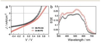
Fig. 7 (a) J-V characteristics and (b) EQE of bulk-heterojunction solar cells containing MI-PO-C8 or Di-MI-PO as the electron acceptor and P3HT as the electron donor.
